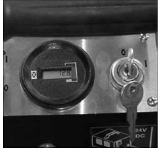
The Wrangler 2016 is available with a Key-And-Hour-Meter option. The key increases safety, preventing unauthorized operation. The Hour Meter makes it easy to track runtimes for routine maintenance procedures.
