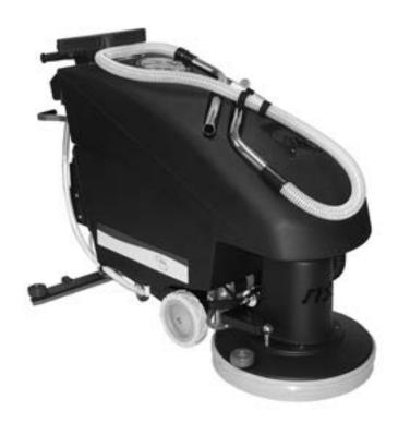
A tight turning radius and scrub head lock-down feature allow the mid-sized Wrangler 2016 to tackle heavy scrub and standard scrub jobs with ease. Its 20-in. scrubbing path makes quick work of any task. A rugged, rotocast-polyethylene body and 7-gauge steel frame deliver long term durability.
