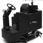
The Champ 3529 is available with an optional Industrial Kit, which includes a headlight, an overhead flashing light and a bumper (not shown).
